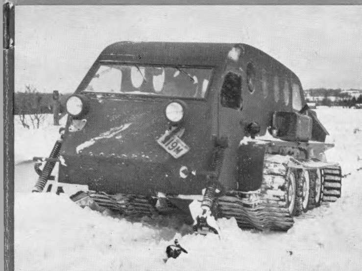
SNOWMOBILE —Newest model in the General Motors War Fashion Parade. Not as streamlined as some but capable of moving men or supplies through deep snow and slush. Caterpillar treads make easy going of rough country.
